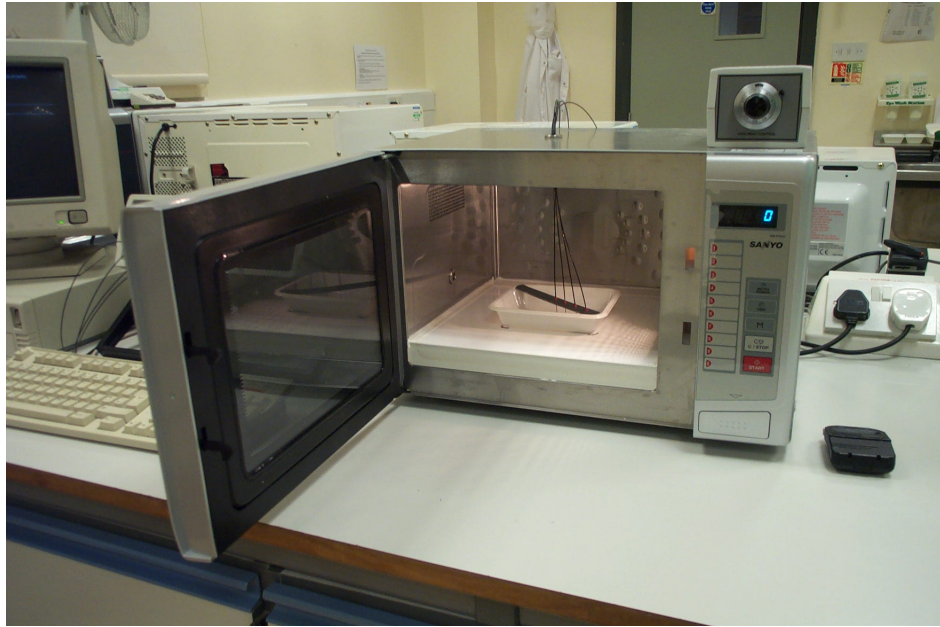
Figure 2: A mode stirred microwave oven showing the food tray and the temperature probes
