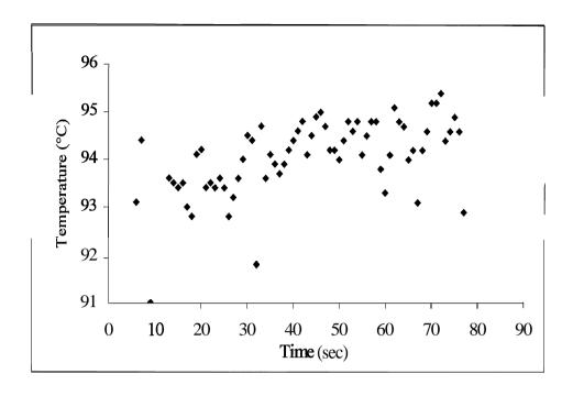
Figure 13. Temperature distribution in a stirred vessel containing 200 L of 5 wt % Colflo 67 starch solution controlled at 94 °C.
