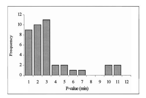
Figure 12. Chart showing distribution of P-values for 42 TTI particles processed in 200 L of 5 wt% Colflo 67 starch solution.
