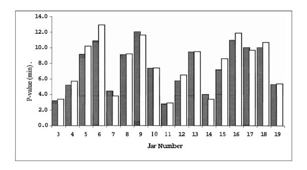
Figure 15. P-values measured for pickled cucumber slices, with two TTIs in one slice of cucumber in the centre of each jar.
