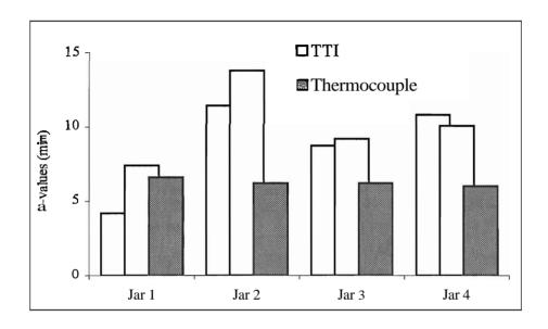
Figure 11. Run 2 results from validation tests between TTIs and thermocouples processed in jars of water in a water bath.
