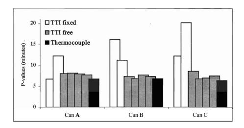
Figure 9. P-values measured by thermocouples and TTIs in cans of water processed with end-over-endrotation.
