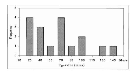
Figure 17. Frequency of P-values measured by B *lichenifomis* in a fruit preparation processed by ohmic heating with a flow rate of approximately 815-850 kg/h.
