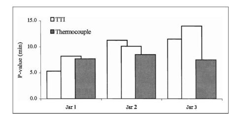
Figure 10. Run 1 results from validation tests carried out in jars of water with TTIs and thermocouples measuring the process lethality.
