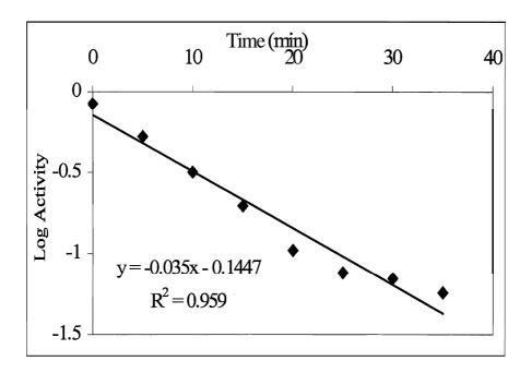
Figure 2. Effect of heating B. amyloliquefaciens amylase at 79 °C on the enzyme activity.
