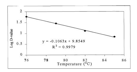
Figure 5. Effect of heating temperature on the D-value of B. amyloliquefaciens amylase.
