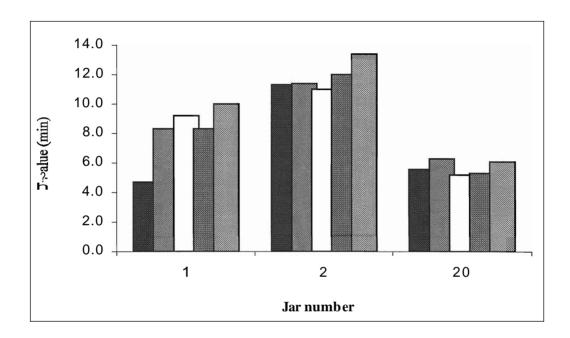
Figure 14. P-values measured for sliced pickled cucumber, with TTIs in Jars 1 and 2 in different slices within the jar, and 5 TTIs in Jar 20 in one slice in the jar centre.
