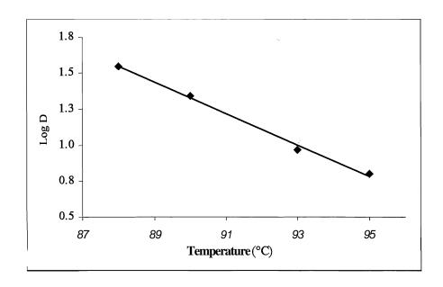
Figure 7. Effect of heating temperature on the D-value for inactivation of B. licheniformis amylase.
