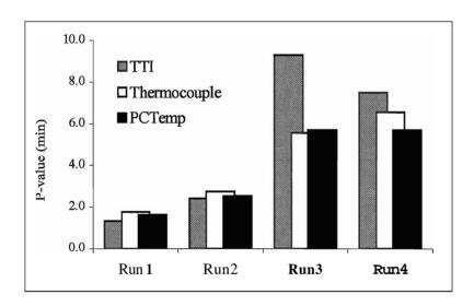
Figure 8. Comparison of P-values calculated from thermocouples and TTIs from trials in a stirred water bath.
