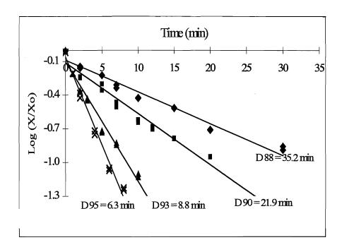
Figure 6. Effect of heating B. *amyloliquefaciens* amylase in the temperature range 88 – 95°C on the enzyme activity.
